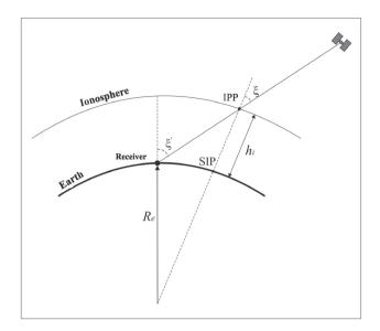
Figure 1. Trigonometric single-layer mapping function (Davies and Hartmann, 1997).
