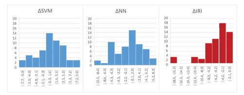
Figure 7. Histograms of the differences between actual and modeled TEC values for best performing SVM and NN techniques and for global IRI model.
