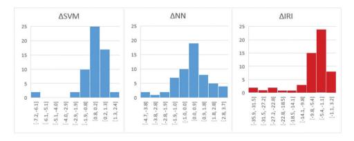
Figure 8. Histograms of the differences between actual and modelled TEC values for best performing SVM and NN techniques and for global IRI model.
