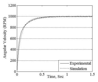
**Figure 4.** The experimental and simulation angular velocities for Example 1.
