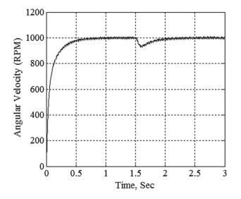
Figure 6. The load torque effect for Example 1.
