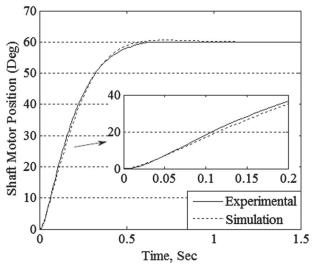
**Figure 8.** The experimental and simulation motor shaft positions for Example 2.
