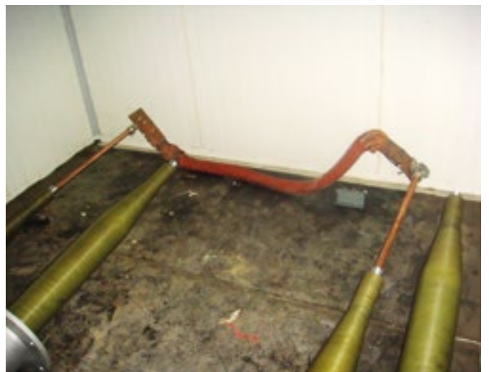
Figure 7. Low temperature test with current injected
