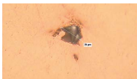
Figure 12. A 26 µm hole in the inner surface
