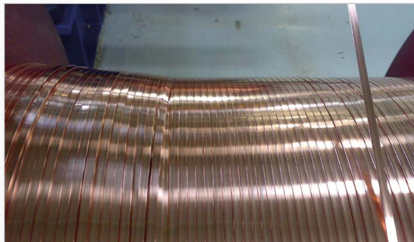
Figure 5. Flat bare strip after the flat rolling stage
