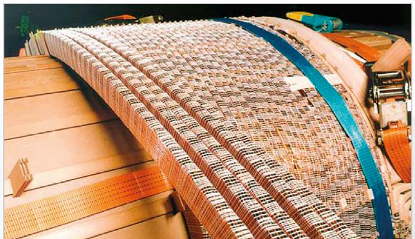
Figure 8. Netting-taped CTC after transposing
