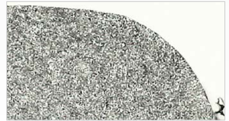
Figure 24. Grain size of a Cu-strip: 10-15 \mu\text{m} (cross-section with corner radius)
