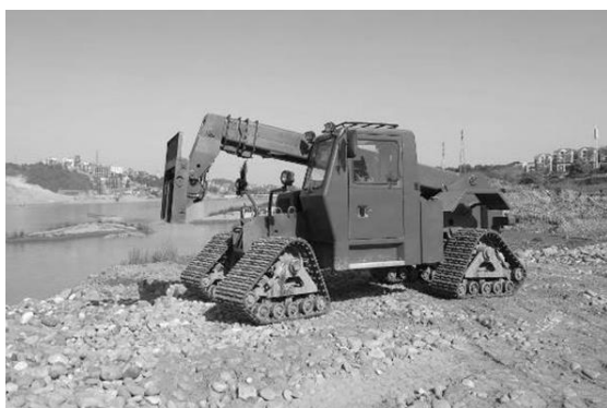
b) After the vehicle equipped with rubber track system
