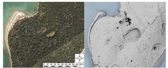
Fig. 11: Left: Orthophoto of the area showing dense Mediterranean vegetation. Right: ALS-derived DTM after archaeological filtering showing the church of Saint Platon. ©LBI ArchPro
