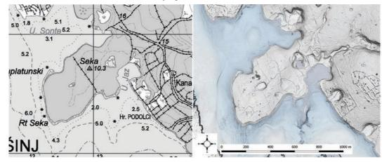
Fig. 10: A comparison of the topographic map (left) and the digital terrain model which is cleared of vegetation (right) and shows many more features in the landscape in a more detailed level. ©Left: Državna geodetska uprava Republike Hrvatske. Right: LBI ArchPro.
