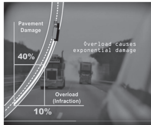
Figure 5 – Relationship of the vehicle overload and the damage to the carriageway
