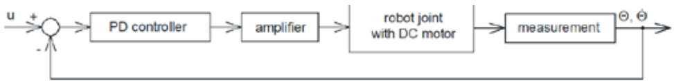
Figure 4. The scheme of the 2nd order system of the inner control of robot joint with motor.
