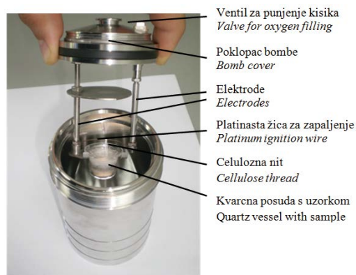
Slika 1. Priprema kalorimeterske bombe Figure 1. Preparation of a calorimeter bomb
