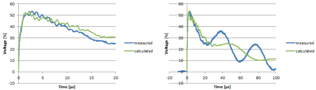
**Figure 5 - Comparison of the simulation and measured results for the cast-resin Resibloc<sup>®</sup>-transformer, top: at winding input, center: layer-to-layer insulation, bottom: section-to-section-insulation.**
