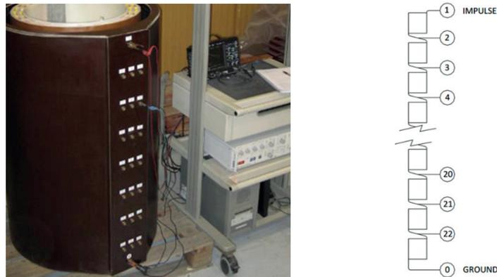
**Figure 6 – Test arrangement (left) and HV measuring taps for the dry-type 1600 kVA transformer (right)**
