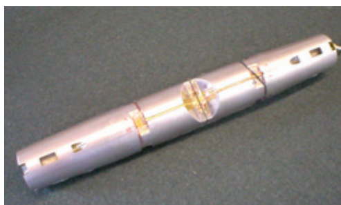
Figure 5 Five-component wind tunnel balance with foil strain gauges
