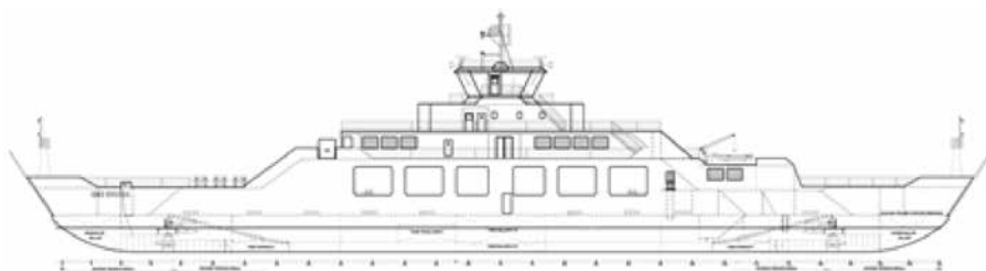
Figure 7: General arrangement of the analysed Ro-Ro passenger ship
