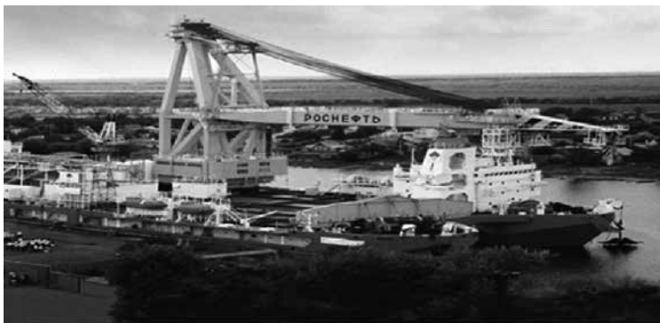
Figure 7 Catamaran crane of 12000 kN lifting capacity
