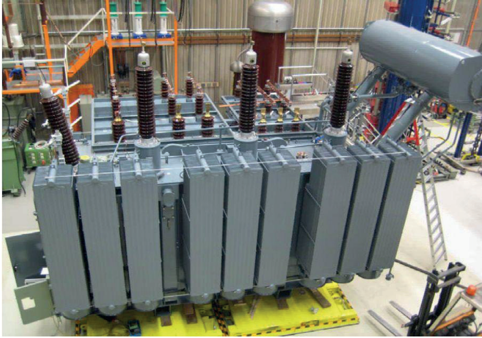
Figure 1 – Prototype transformer with ONAN / ONAF cooling in test field
