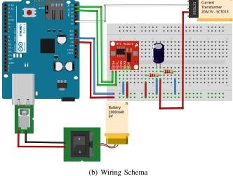
Figure 1. Connections of the single-phase collector device and Wiring
