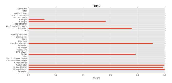
Figure 9. Accuracy of FHMM algorithm.
