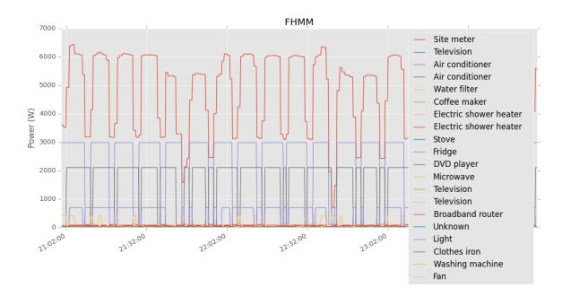
Figure 6. Disaggregation plot by FHMM algorithm.
