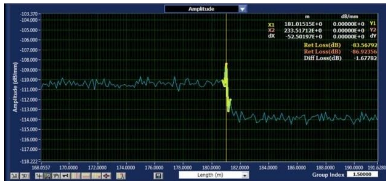
Fig. 2. Example signal from Luna optical backscatter reflectometer
