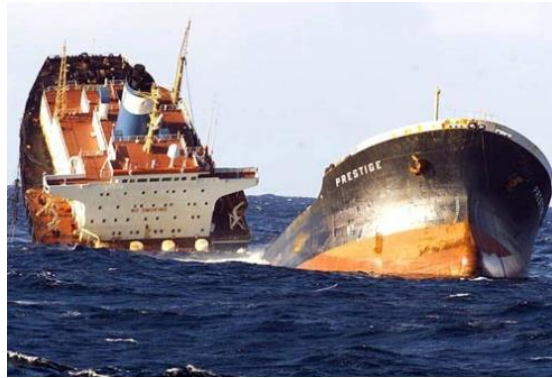
Fig. 1. A maritime disaster resulted from the collapse of the hull structure [ http://portalmarynarski.pl ]
