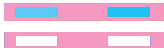
Figure 2. Test sample of the crispening effect with the secondary stimulus of 50% RTV and the primary stimuli of 55% RTV (left) and 65% RTV (right)
