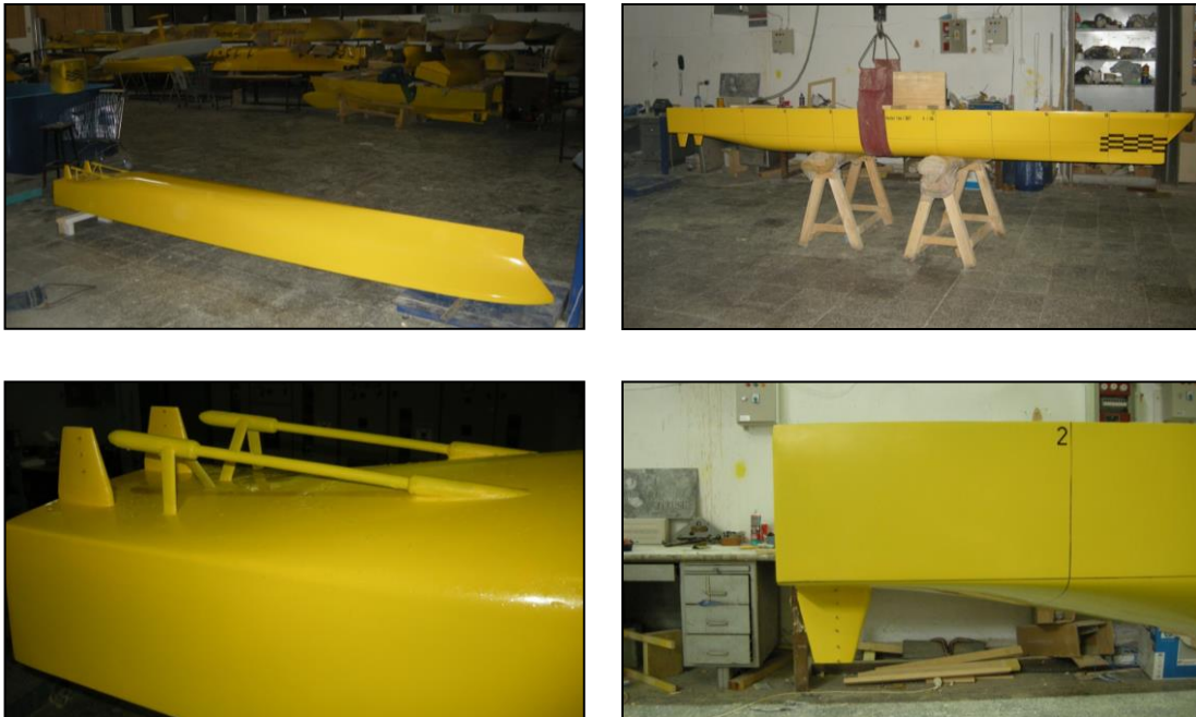
Fig. 2 Different views of the M367 ship model with and without appendages
