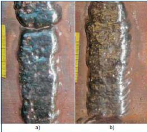
Slika 9. Prikaz lica zavara na vratu uzoraka 3 (a) i 5 (b) Figure 9. Appearance of weld face on rail neck on samples 3 a) and 5 b)
