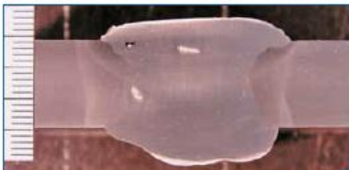
Slika 13. Makroizbrusak nožice tračnice uzorka 5 Figure 13. Macrosection of rail foot weld on sample 5
