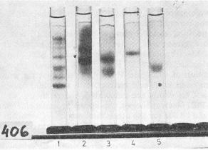
Figure 3. Polyacrylamide gel electrophoresis at pH 4.4 of enzymes at various purification steps. Gel 1: ammonium sulphate fraction; gel 2: Sephadex G-75 concentrate; gel 3: the second peak from thiol Sepharose; gel 4: cathepsin B (the first maximum from CM-cellulose); gel 5: CM II (the second maximum from CM-cellulose).
