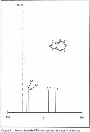
azulene (\_\_\_\_\_) and of enriched azulene from the synthetic route in Scheme II (\_\_\_\_\_\_).
