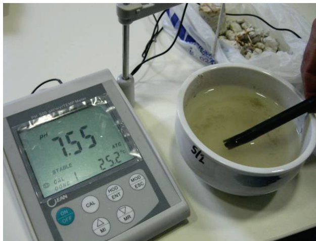
Figure 7 Measuring the pH-value of a concrete sample from synagogue in Subotica
