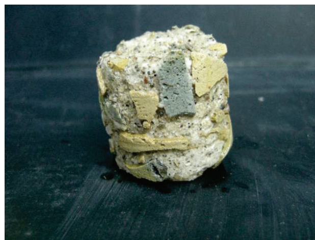
Figure 4 Sample from the concrete vault of the Subotica synagogue with a coarse crushed fired clay aggregate and gypsum, which partly dissolved in water
