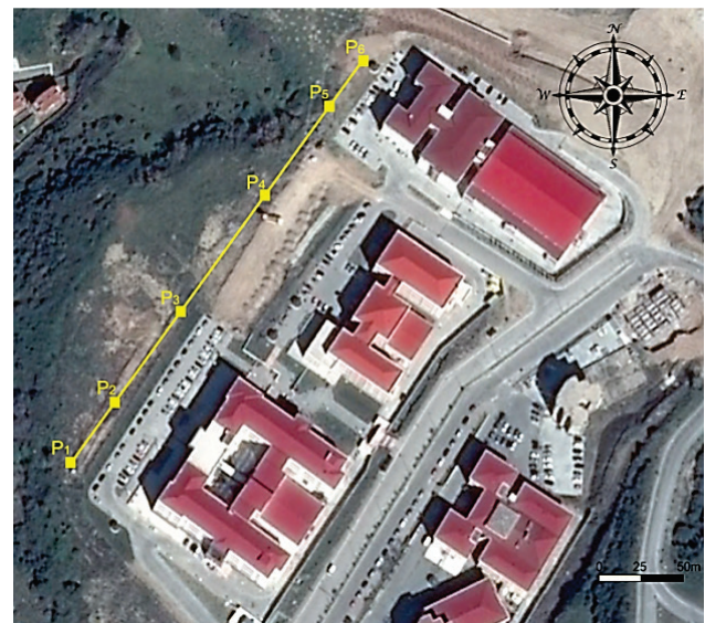
Figure 7 The benchmarks and baselines in Terzioglu Campus
