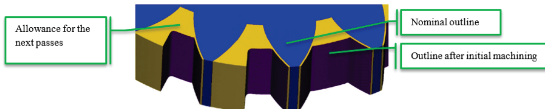
Figure 7 Example of space machining sequence. On the left: two spaces machined on one side of a tooth. On the right: one full space machined to the predetermined depth. Yellow colour – the remaining allowance
