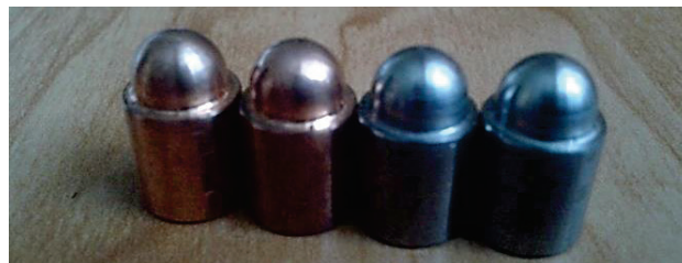
Figure 3 Photos of hemisphere samples from copper and steel
