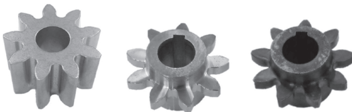
Fig. 2 Sintered gear after compaction and sintering (left), after machining (middle) and after heat treatment (right)
