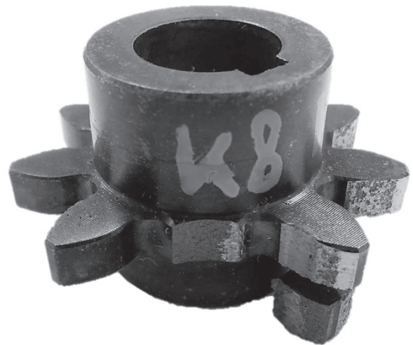
Fig. 8 Typical damage after test – test gear K08
