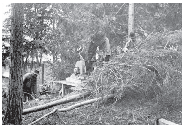
Fig. 1 In times of disturbances to international trade and threatening isolation, such as the great wars, efforts were made to modernize and intensify the use of forest biomass for energy in the Nordic countries. The picture shows chunking of coniferous branchwood with the manually driven smallwood chunker »Ursus« in a south Swedish forest at the time of the First World War (from Nilsson 2016)
