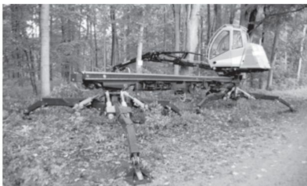
Fig. 6 The Portaltharvester, with its two tripod legs and sliding cab (Photo courtesy of Christian Knobloch)
