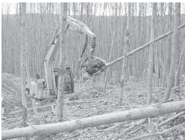
Fig. 2 Mechanized cut-to-length harvesting in a chestnut coppice
