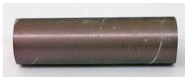
Figure 3 Photo of the sample 14. Is visible the grey oxide deposited on the specimen surface.
