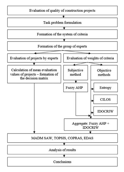
Figure 1. The scheme for evaluation of the quality of construction projects. Source: Created by the authors.
