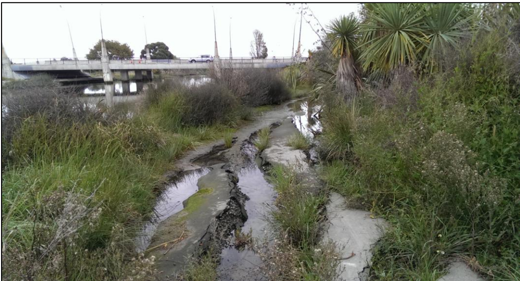
Figure 4. Ground deformation and subsidence caused by the Canterbury earthquakes.
