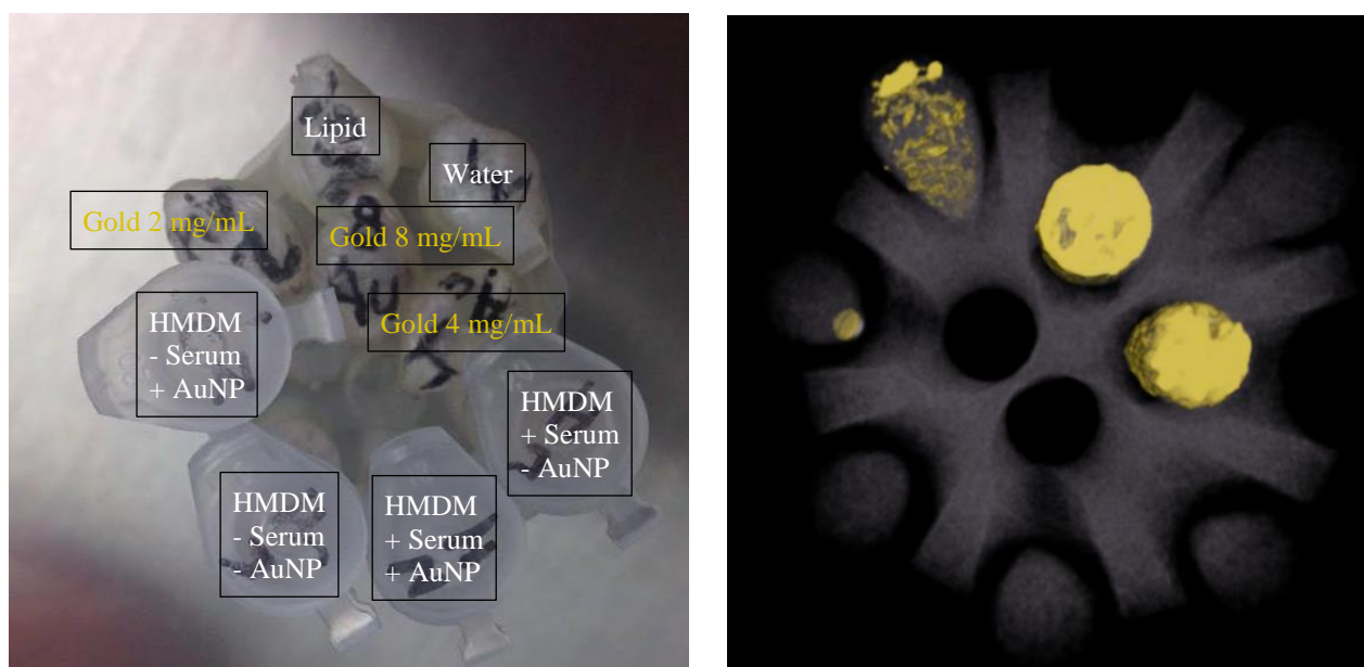
Figure 8.5 Photo of layout of vials (left) and MARS image (right) of macrophages with non-functionalized gold nanoparticles.
