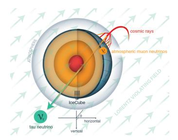
FIG. 1: Schematic figure of the test of LV with atmospheric neutrinos in IceCube. Muon neutrinos produced in the upper atmosphere are detected by IceCube in Antarctica. The potential signal is the anomalous disappearance of muon neutrinos, which might be caused by the presence of a hypothetical LV field that permeates space. The effect can be directional (arrows), but in this analysis we test the isotropic component.
