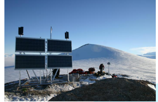
Small scale solar panels can generate electrical energy to power small devices either out in the field or at national bases. Credit http://adam.antarcticanz.govt.nz
