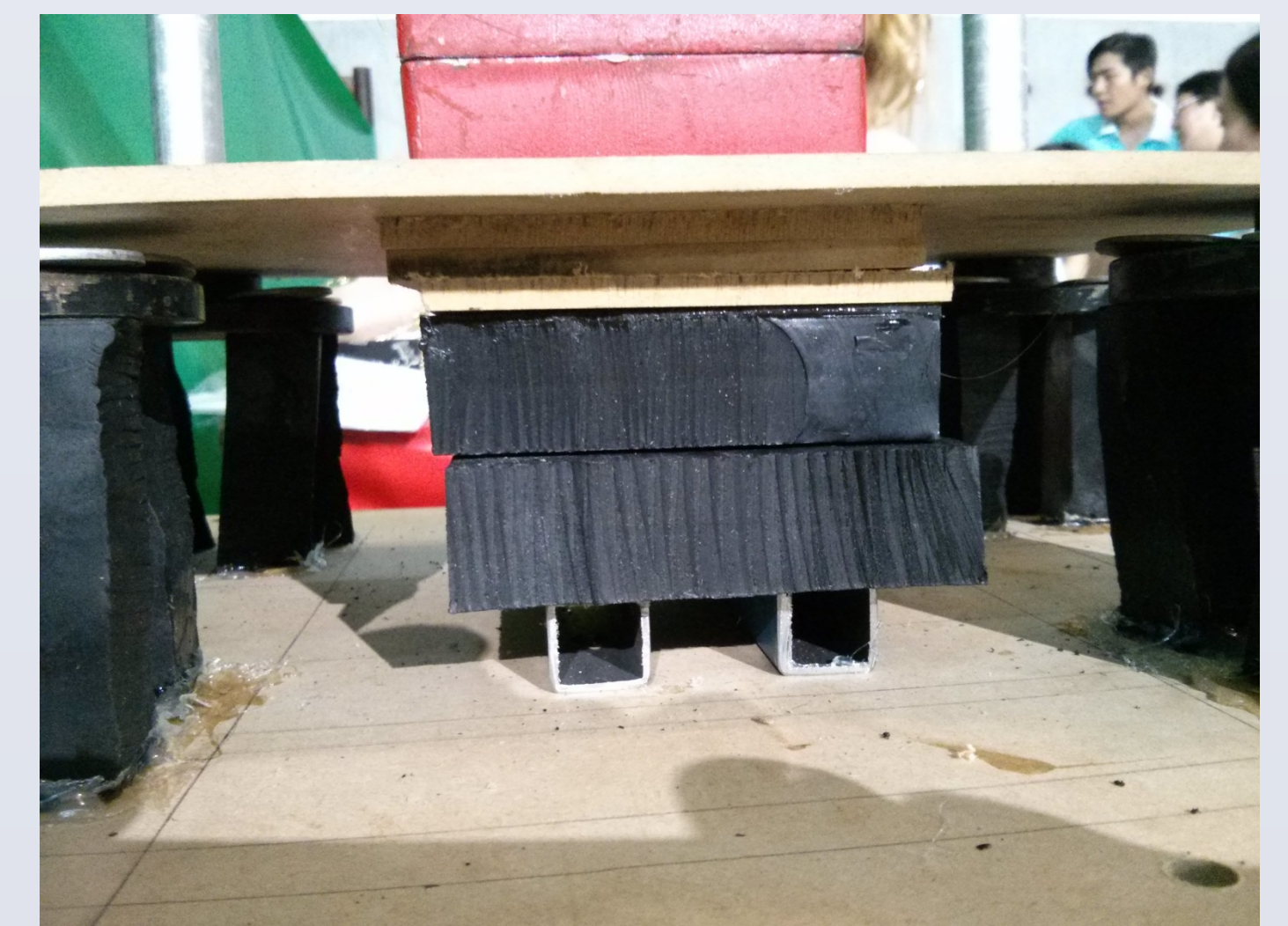
Base isolators and friction damper at the base level
