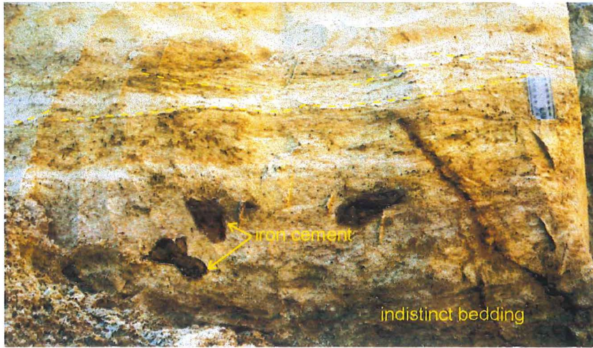
a: Iron cement blobs, indistinct and wavy bedding and cross bedding in McLaughlins Quarry. F12P4.
