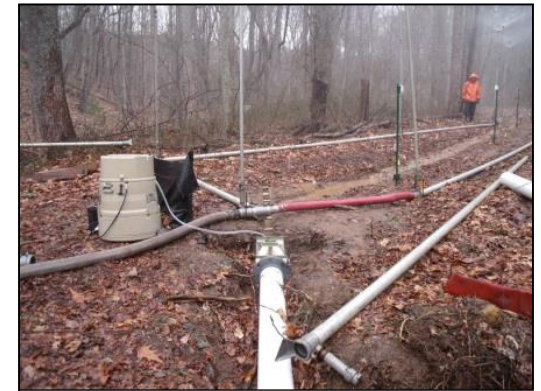
1" X 18" cutthroat flume and ISCO stormwater sampler
