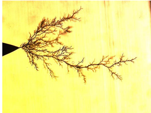
Figure 2.5: An example of electrical treeing in power transformer insulation ( Treeing ).
