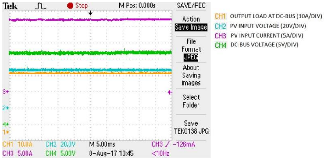
Figure 5-20. MPPT mode of PV channel at the 1 kW MPP
