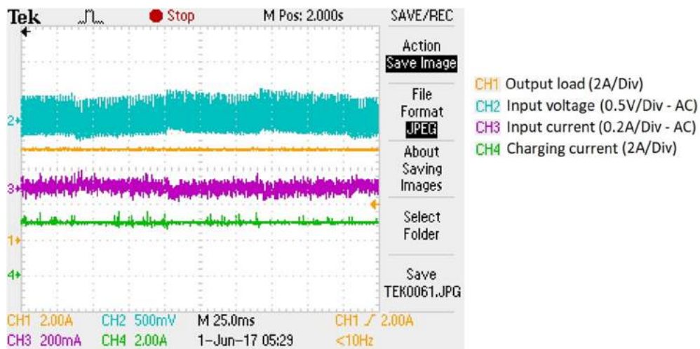
Figure 5-19. MPPT mode is operating around the maximum power point for PV input
