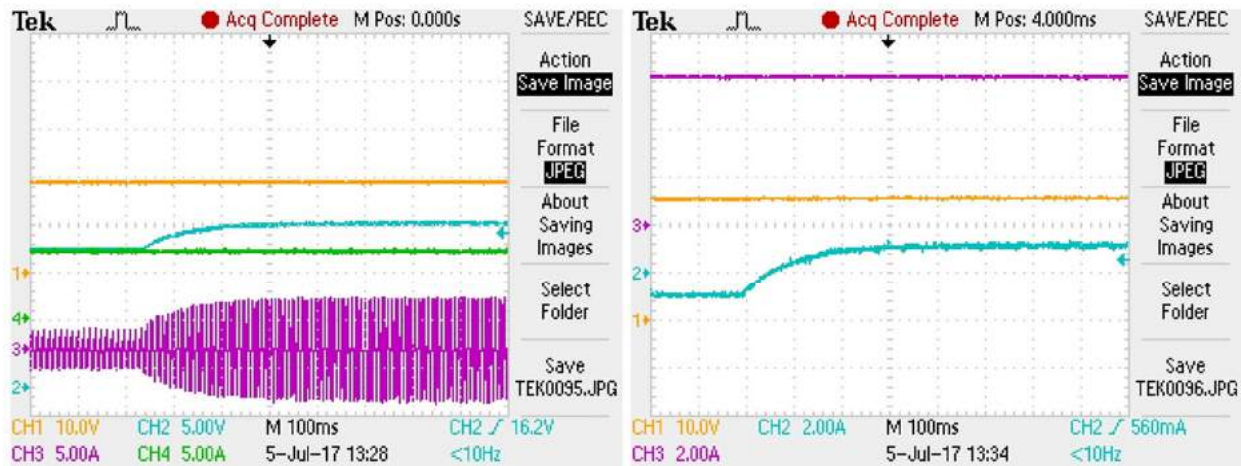
a) INPUTS WAVEFORMS CH1: PV VOLTAGE, CH2: TB VOLTAGE (RECTIFIED DC) CH3: TB CURRENT (ON PHASE A), CH4: PV CURRENT
