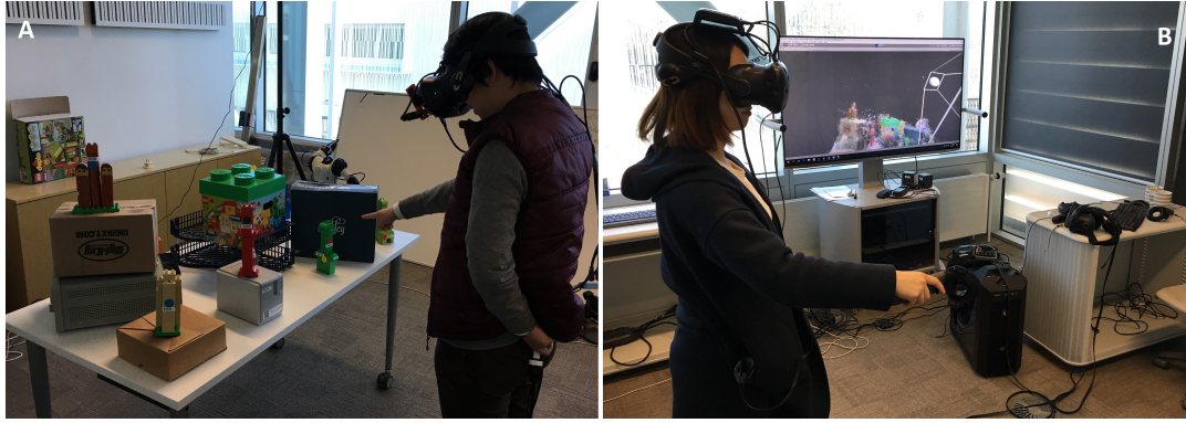
Figure 1: Static local environment capturing with real-time feedback for Mixed Reality remote collaboration. A: the local user stands in front of a workspace, identifying a particular LEGO model which the remote helper has pointed at. B: The remote expert observes the local environment and guides local worker via pointing in the VR world.
