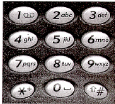
Fig. 1.2: A standard ISO 12-key keypad as found on the Nokia 5110.
