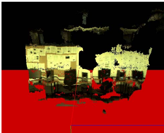
Figure 1: Disparity data from a simple scene with the calculated ground plane superimposed as a red region.
