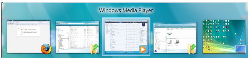
(b) Vista A1t+Tab displaying thumbnails. The active selection has a highlight border around its thumbnail, and a title displayed above the thumbnail list.
