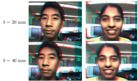
Figure 2.3.7. Comparison between two different camera separation for a handheld device. (Mangiate 2012)
