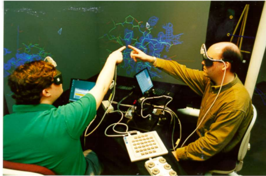
Figure 2.2.3. Physical separation for multiple users. Each user has his/her own physical screen but they share the visualization (Arthur 1998).
