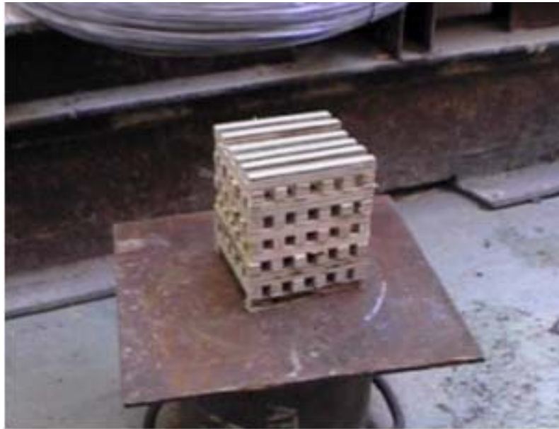
Figure 30 - Typical wood crib
