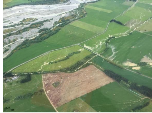
Figure 48: Standing water and ejecta west of Waiau town (-42.638°, 172.993°).
