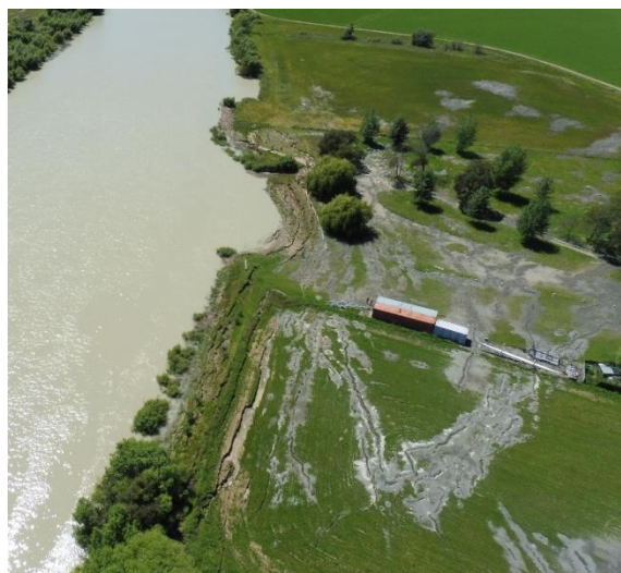
Figure 22: Aerial view of liquefaction manifestation at the Blenheim Rowing Club (Approx. coord: -41.4882^{\circ} , 174.0100^{\circ} , taken facing E). Photo: Marlborough District Council.
