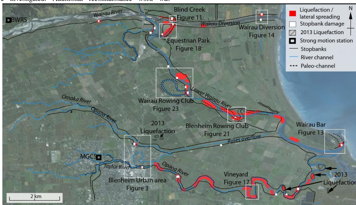
Figure 2: Overview of liquefaction damage in Blenheim and the Wairau Plains resulting from the 2016 M_w7.8 Kaikōura earthquake and 2013 M_w6.6 Lake Grassmere earthquake (Approx. coord. of centre of image: -41.495^\circ , 173.980^\circ ).
