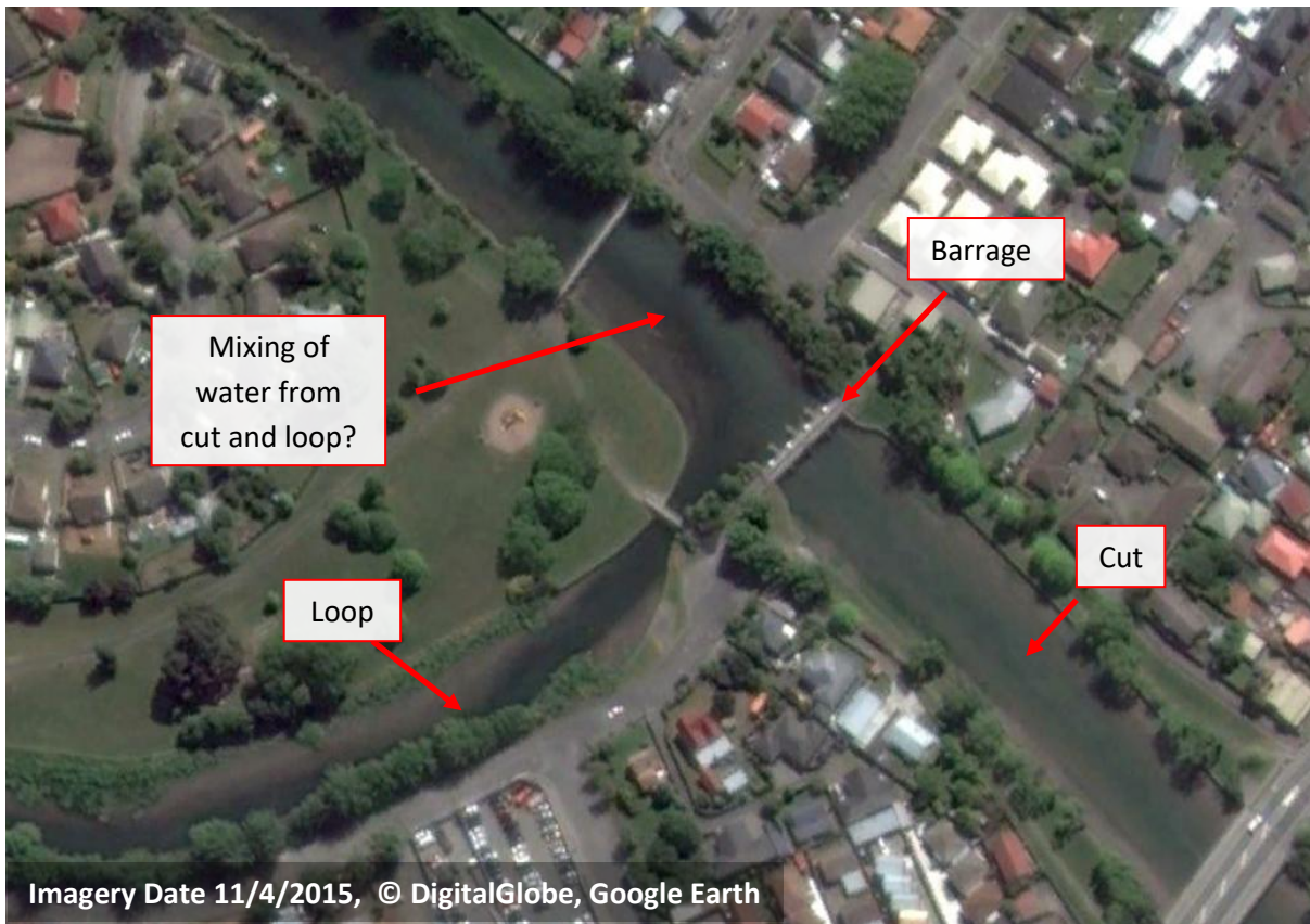
Figure 8. Aerial photo appearing to show leakage of lighter coloured estuarine water upstream through Woolston Barrage on incoming tide in April 2015.
