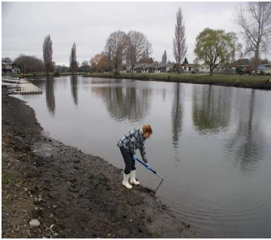
c) Sampling at Kerrs Reach. Note the high level of sedimentation due to liquefaction generated by earthquakes
