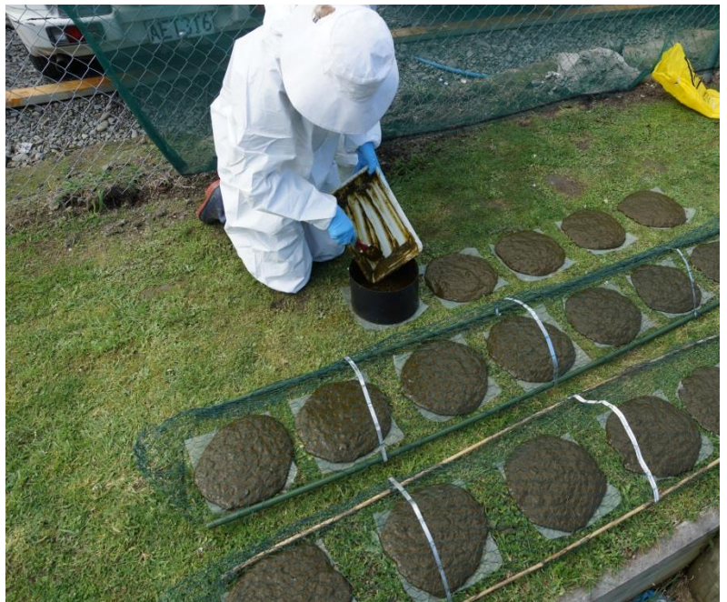
Pouring weighed 1kg of cow faeces into sterile ring for simulated cowpats
