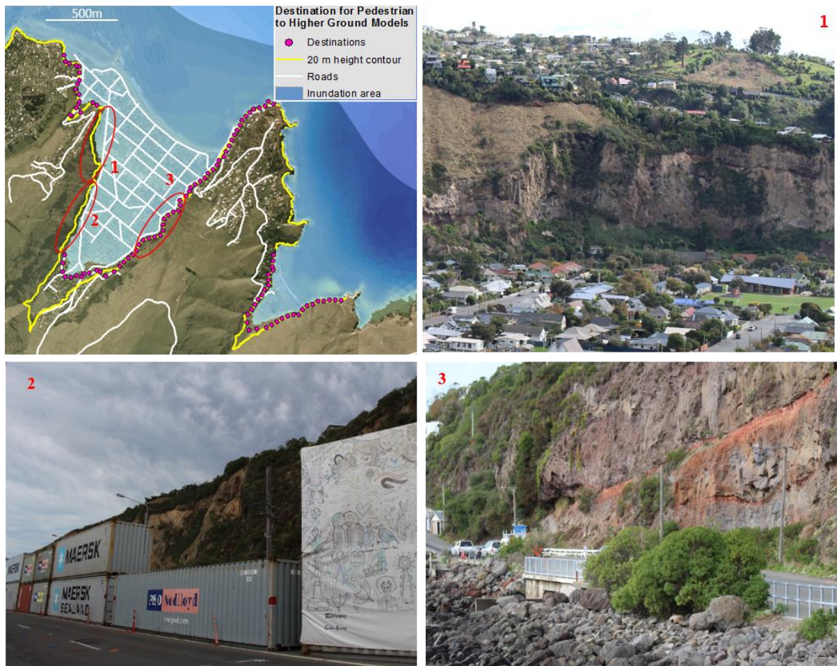
Figure 3.10. (Top-left) Destinations for pedestrian evacuation to higher ground. The total number of Destinations is 105 points; (Top-right) Photo shows steep slopes on Wakefield Road, numbered 1 in the destinations map (May, 2015); (Bottom-left) Photo shows rock fall protection containers on Wakefield Avenue, numbered 2 in the destinations map (May, 2015); (Bottom-right) Photo shows steep slopes on the other side of the valley, chosen to be destinations in model – these points were kept as destinations within the model to test whether or not the model would evacuate people to these unrealistic locations, numbered 3 in the destination maps (May, 2016).
