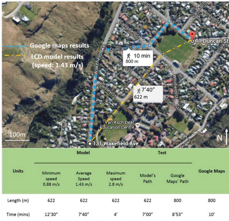
Figure 3.22. The map shows results for evacuation on relatively flat landscape to bus stop on Duncan Street by LCD model and Google Maps; The table shows details results by LCD model (minimum, average, and maximum speed), real-life test on model's Path and Google Maps' Path, and Google Maps.
